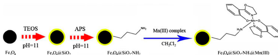
Scheme 1. Step-by-step synthesis of \text{Fe}_3\text{O}_4@\text{SiO}_2\text{-NH}_2@\text{Mn(III)} .
